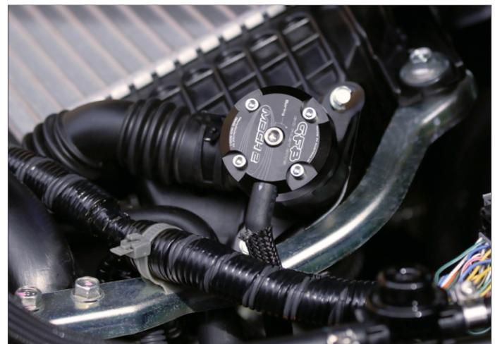
5) Replace the two bolts, vacuum and recirc hoses and clamps.
